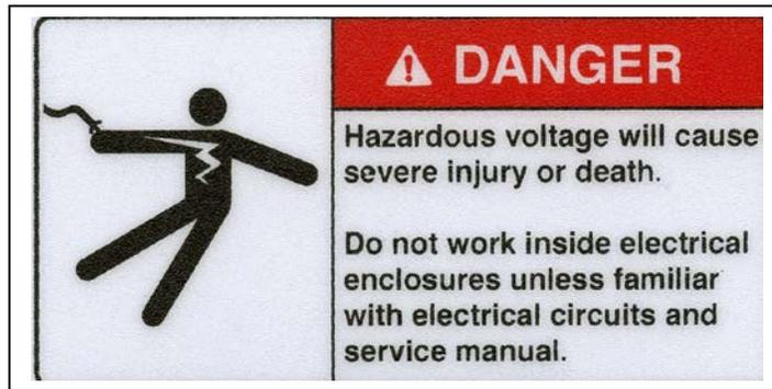
This label is located on printing units, folders, and rollstands equipped with electrical devices, as well as press drive. It alerts the operator of the danger of electric shock that could cause severe injury or death if the devices or wiring is entered for service or repair. It also warns the operator to call a qualified electrician to perform any electrical repairs on the unit to avoid personal injury.
